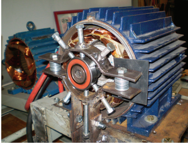
Fig. 14. Eccentricity induced failure
